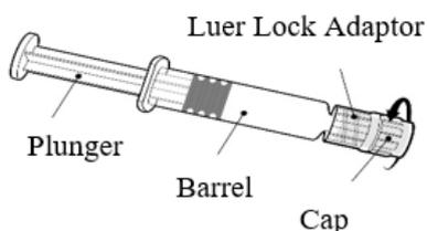
Hold the syringe by the barrel and not the plunger.
